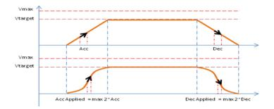
As can be seen in the graph, without the application of the JerkRatio, the Acceleration / Deceleration is at the configured Acceleration / Deceleration. When the JerkRatio is applied however, the Acceleration / Deceleration may be affected by as much as two times that of the configured Acceleration / Deceleration value.
